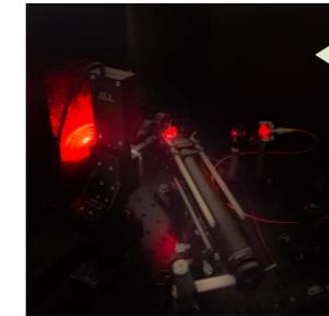
Our LIDT measurement set-up is fully automated, from the laser control to the diffusion-based damage counting. This way, we ensure perfect repeatability for every test.
