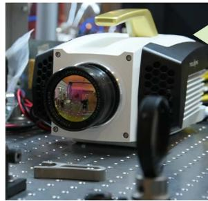
We are equipped with high resolution, high speed thermal cameras (up to 14 kHz frame rate) that can accurately evaluate the origin of unwanted thermo-optical effects.
