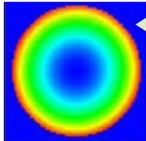
Optics with unknown radius of curvature can be accurately measured, whether convex or concave, from 2 to 50 m, for optics from 10 to 30 mm diameter.
