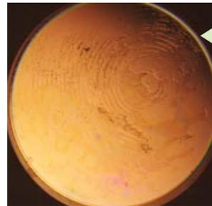
Presence of dust, organic contaminants, scratches and digs of an optical surface can be evaluated, preventing potential damages during high power laser operation.
