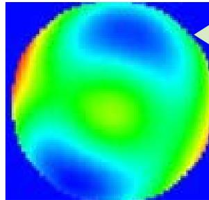
The transmitted wavefront error (TWE) of an optic can be evaluated on a large surface (up to 25 mm diameter), with a precision down to  $\lambda/20$  at 633 nm.
