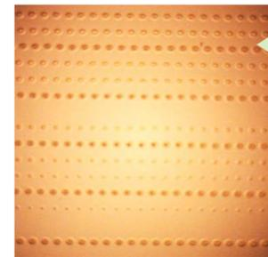
We provide standardized LIDT tests based on ISO-21254. Optics from different manufacturers can be easily compared to select the most resistant one.
