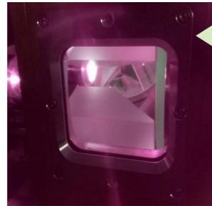
We systematically test our opto-mechanical systems in dedicated test benches, measuring key parameters such as the thermo-mechanically induced wavefront error, long term pointing stability.
