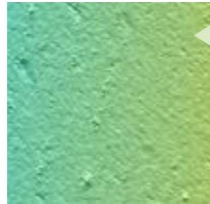
Precise surface roughness down to few nanometers can be easily measured with optical profilometry.
