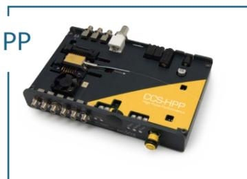
➤ Open driver for HPP (High Pulse Performance) electronic Board
