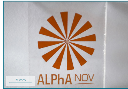
Intra-volume colouring of a doped glass
