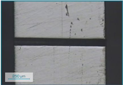
Stainless steel drilling - cross section
