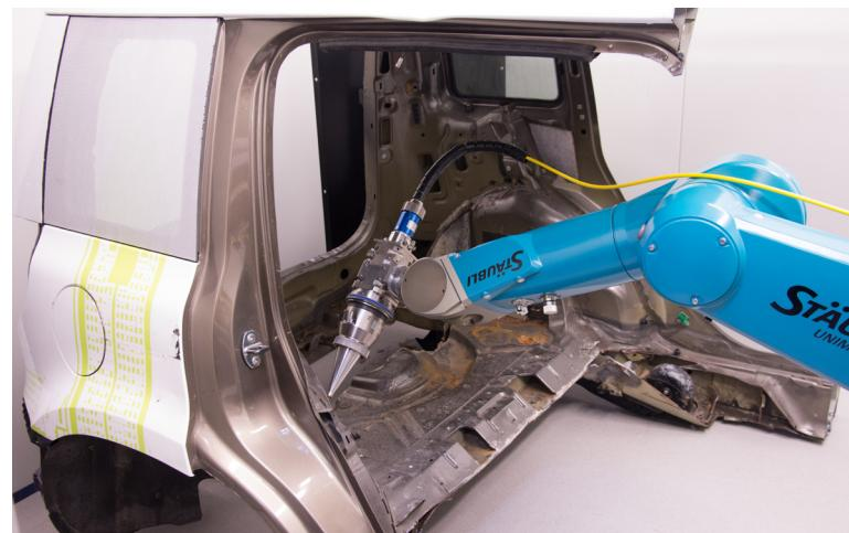
Laser system for micromachining
