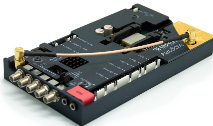
Figure 8 : Shaper board for EOM driving, combining a laser diode driver, a multiple output synchronization electronics and a 5V programmable shape output to drive an EOM with 2GHz bandwidth and 48dB dynamic range
