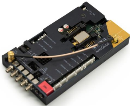
Figure 14 : AeroDIODE shaper module set in direct driver configuration (left) and special optical pulse shape obtained from a DFB laser diode after its programmed within the module (right)
