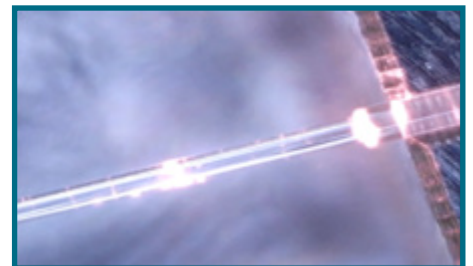
Picture of a CO 2 laser splice between a fiber bundle and the output active fiber
