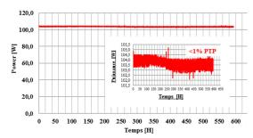
Laser stability over 3 weeks of continuous burn in at 100 W/100 kW peak power
